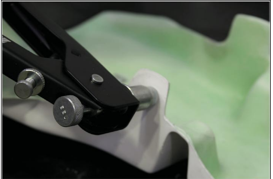
Rivnuts are similar to a rivet but they have a captive nut inside them and are very handy for fixing lower tails to upper tails and sometimes even frame mounting.
