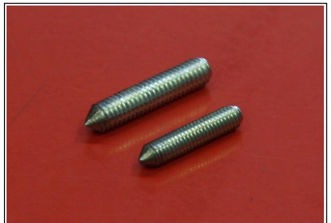
Get a spare 6mm and 5mm bolt, cut the head off and use a grinder to taper the bolt head end to a point.
