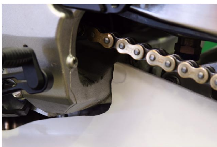
Sometimes you may need to grind areas of the fairing so that they fit around corners/over edges.
