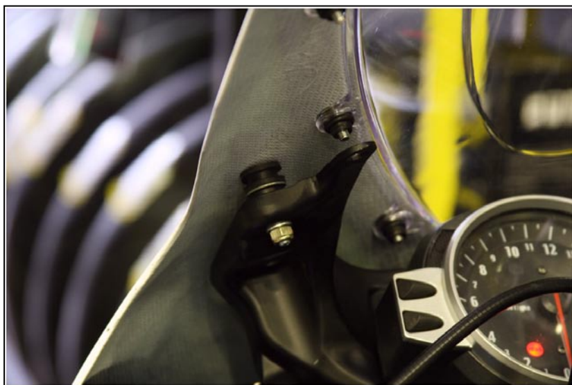
Here is an example of an upper fairing not aligning with a slightly twisted stay bracket. A simple solution was to install a spacer and mount the upper fairing off the bracket.
