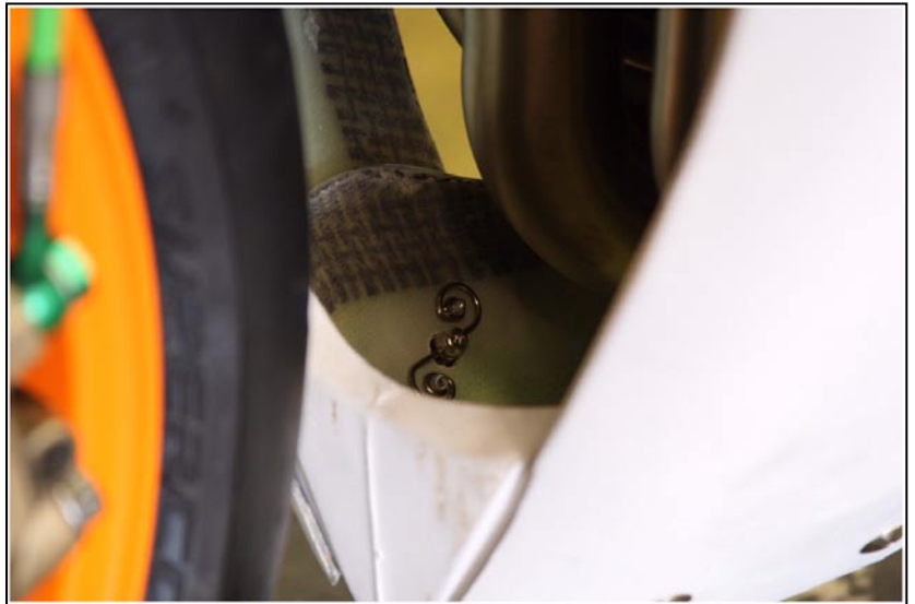
Dzus Fasteners are great for connecting upper and lower fairings.
