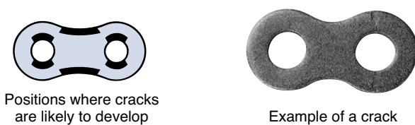
Fig. 23 Cracks on the link plates
