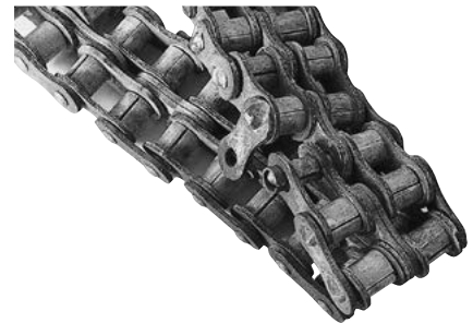
Fig. 31 Corrosion of stainless steel roller chain
