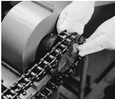
Fig. 8 Connecting on a sprocket
