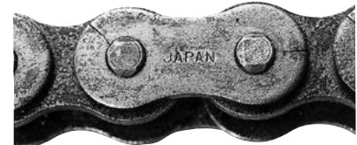
Fig. 32 Hydrogen embrittlement cracking
