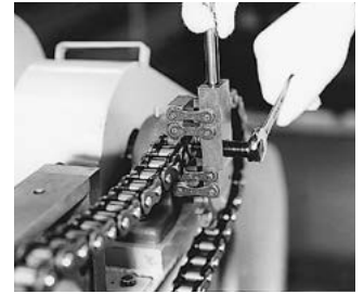
Fig. 5 How to cut a chain using a chain screw
