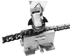
Fig. 2 Grinding the pin ends
