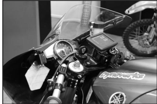
Pic 4. High Mount is better for GPS signal reception and use with the Basic System (no external GPS).
