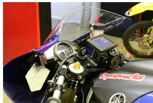
Pic 4. High mount is better for GPS Signal reception and for use with RaceChrono Basic (no external GPS).
